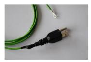
In order to attach the grounding cable to your STEPCRAFT CNC machine, please remove the screw either on the left or on the right side of the control bar on the control retaining plate. Onto this screw you firstly slip the eyelet of the grounding cable, then the serrated lock washer. Now, please reattach the screw to the place at the control retaining plate where it has been removed.
